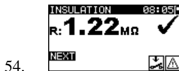
Figure 0.75: Insulation result screen
