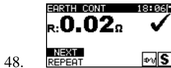
Figure 0.73: Earth continuity result screen
