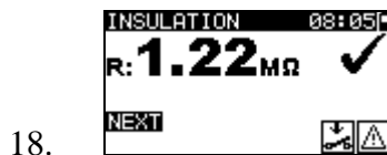
Figure 0.59: VDE Organizer – Insulation resistance result screen
