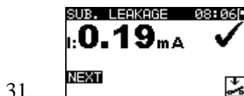
Figure 0.61: VDE Organizer – Substitute leakage result screen
