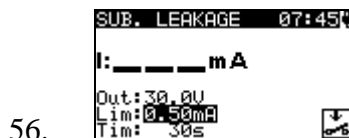
Figure 0.76: Substitute leakage starting screen
