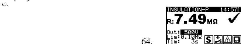
Figure 0.79: Insulation resistance - P result screen
