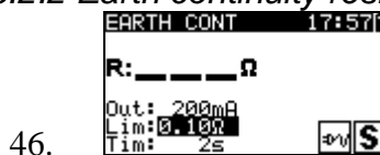
Figure 0.72: Earth continuity starting screen
