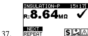
Figure 0.63: VDE Organizer – Insulation resistance - P result screen
