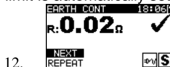
Figure 0.57: VDE Organizer – Earth continuity result screen
