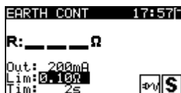
Figure 0.31: Example of single test measuring menu
