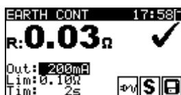
Figure 0.35: Examples of Earth continuity resistance measurement results
