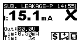
Figure 0.47: Example of substitute leakage - P current measurement results
