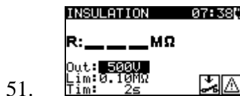
Figure 0.74: Insulation resistance starting screen
