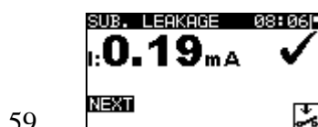
Figure 0.77: Substitute leakage result screen
