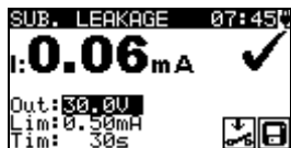
Figure 0.44: Example of substitute leakage current measurement results
