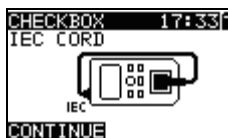
Figure 0.22: IEC test cord check starting screen
