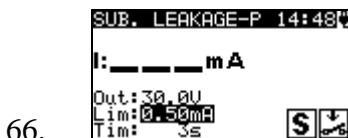
Figure 0.80: Substitute leakage - P starting screen
