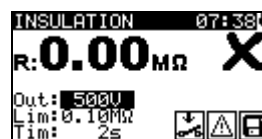
Figure 0.38: Examples of Insulation resistance measurement results
