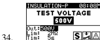
Figure 0.62: VDE Organizer autotest – Insulation resistance - P starting screen
