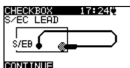
Figure 0.21: S/EB test lead check starting screen
