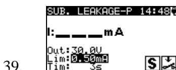
Figure 0.64: VDE Organizer – Substitute leakage - P starting screen
