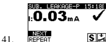
Figure 0.65: VDE Organizer – Substitute leakage - P result screen
